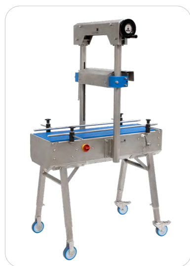
Stand-alone lid pressing roller Wide range adjustable lid pressing roller on a conveyor belt to close the bucket with the lid.
