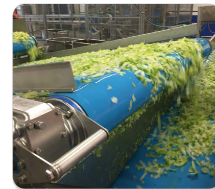
Hygienic conveyor Our hygienic conveyor folds open for very good cleaning.
