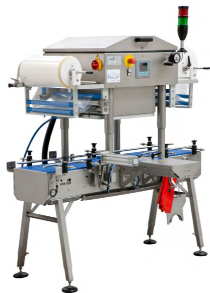
Seal machine Our seal machine on conveyor belt, equipped with dosing-cylinder and position plate. As an option, we can also protect your product by gas filling.
