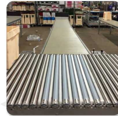
Cross Over This cross-over is designed in a stainless steel frame for the flower-industry with high resistance for dirt, sand and water. Easy to operate, maintain and to clean.
